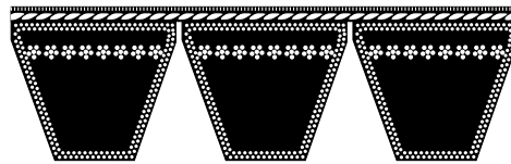
ENVELOPE 5V, 8V CROSS SECTION
